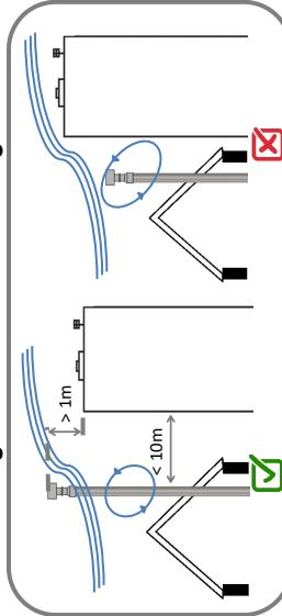
**3º.- Chimney cap installed at the end of the smoke outlet**
