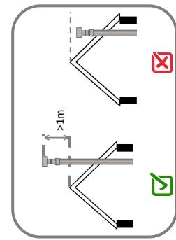
**2º.- Chimney cap above the highest part of the roof ridge but with a taller building close**
